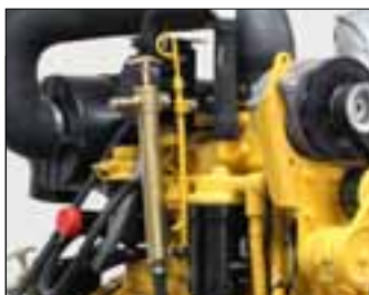
Lube oil drain pump
